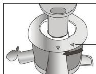
Make sure the lock sign on the hopper and the arrow on the bowl are aligned
